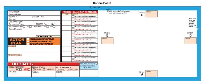
This Incident Command System consists of two tactical command worksheets mounted in a weatherproof case with built in legs. The worksheets have a dry erase surface that accepts magnetic tags that represent the Officers, tasks and apparatus at the incident. The Incident Commander will use the system to track the tactics and assignments throughout the duration of the incident. Custom layouts are available.
